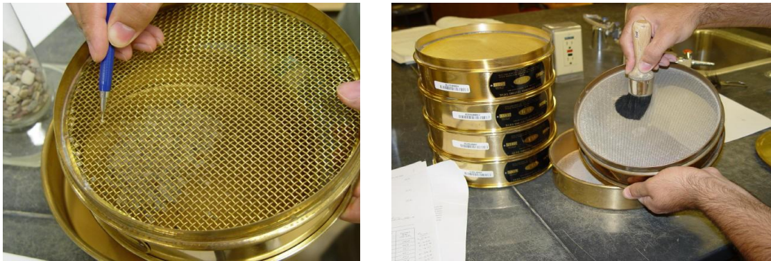
Fig. 7 : Sieve analysis for particle gradation
